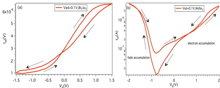
**Figure 6.** Electronic state change verified by transport measurements. Transport characteristics ( $I_{DS} - V_G$ ) of the Bi<sub>2</sub>Se<sub>3</sub> nanoplates (a) and MoSe<sub>2</sub> flakes (b) via the EDL gating effect. Compared to MoSe<sub>2</sub> flakes, the charge transport behavior indicates a heavily n-doped nature of Bi<sub>2</sub>Se<sub>3</sub> nanoplates, such that the Fermi level cannot move into its valence band. The arrows show the direction of the applied voltage sweeps.
