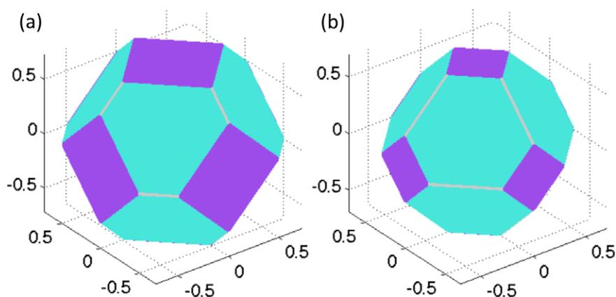
**Figure 2.** The equilibrium particle shape of (a) the ordered structure with a local inverse spinel surface structure with  $\gamma_{\text{total}} = 1.36$  J and (b) the uniformly disordered structure with  $\gamma_{\text{total}} = 1.04$  J. The (100), (110), and (111) facets are depicted using the colors violet, gray, and turquoise, respectively.
