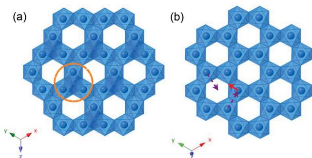
**Figure 6.** Comparison of Mn-distribution between a) the spinel  $\text{LiMn}_2\text{O}_4$  and b) the layered  $\text{Li}_2\text{MnO}_3$  structures. For clarity, only Mn ions are shown. The spinel nucleus is composed of four Mn ions, as indicated by the yellow circle. The red arrow in (b) shows the Mn migration into the Li-layer and two purple arrows suggest a path to increase the range of the spinel nucleus.
