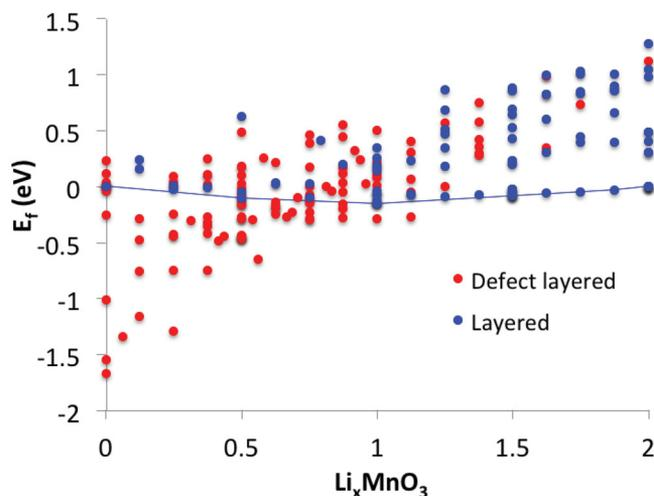
**Figure 2.** The formation (DFT) energy of  $\text{Li}_x\text{MnO}_3$  where the red and blue dots indicate the structures termed defect layered and layered, respectively. The blue line indicates the convex hull of the data sets with layered structures.
