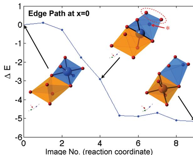
**Figure 5.** The energy profile during a Mn migration via the Edge Path at  $x = 0$ . The points 0 and 9 indicate the initial and final states, respectively. The highlighted oxygen ion (red-star) moves substantially to decrease the distance to the oxygen ions in the red-dashed ellipse.
