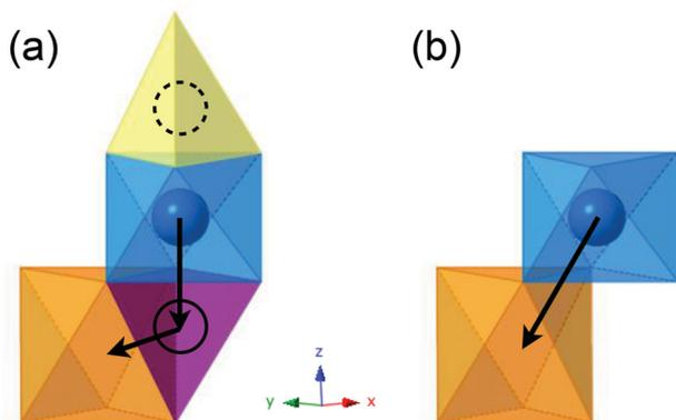
**Figure 4.** Illustration of the two examined paths for Mn migration into the Li-layer: a) the Dumbbell Path, where a dumbbell of Mn (circle)-vacancy-Li (dashed circle) enables a Mn ion at the octahedral site to migrate into the tetrahedral site (purple) and b) the Edge Path.
